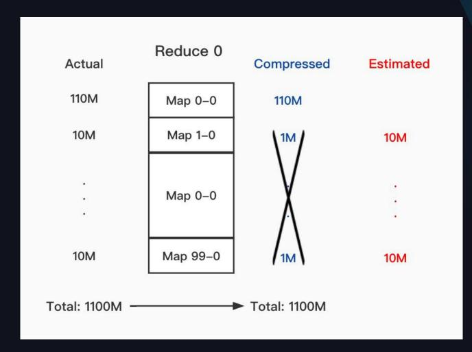
Using the accurate data size of ReduceTask to deduce the corresponding data size of each MapperTask and obtain the more accurate data distribution.
